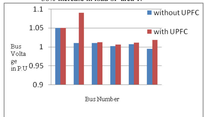
Fig.12. Bus Voltage Profile of Area 1 during generator outage at bus number 2 in area 1 and with 30% increase in load of area 1.
